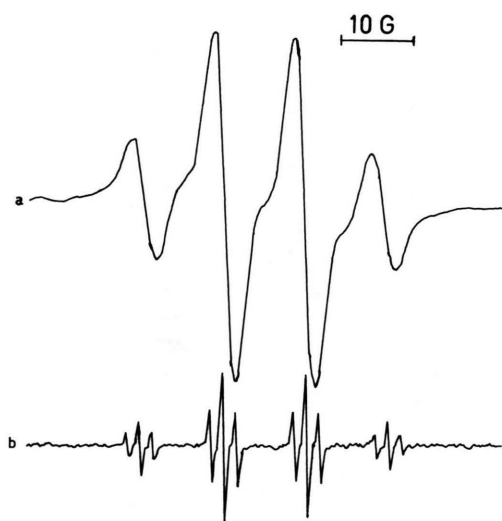
Fig. 2. ESR spectra of gamma irradiated 2,6-di-t-bu-4-methylphenol, a) single crystal, B \parallel c , at 293 K and b) after melting at 353 K.
